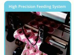
Double mark tracking sensor system to guarantee correct media feeding always.
